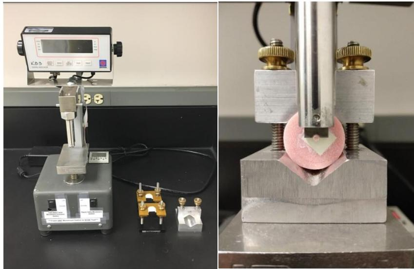
Figure 15 – Top - Ultradent Universal Shear Bond Tester (with sample in place),
