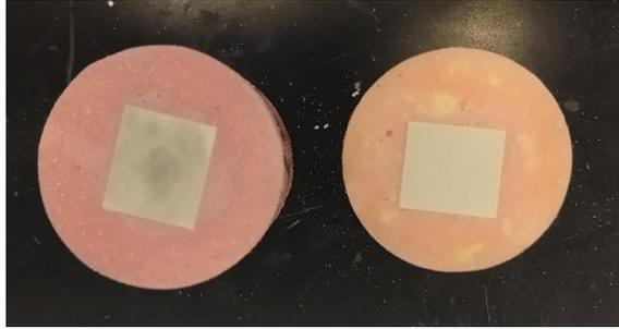
*Figure 18 - Microblasting at 10mm (Left), and 20 mm (Right)*
