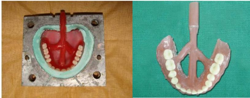
*Figure 9 – Injection molding flask (Left- Sprued denture, Right - Processed denture with sprue attached)*
