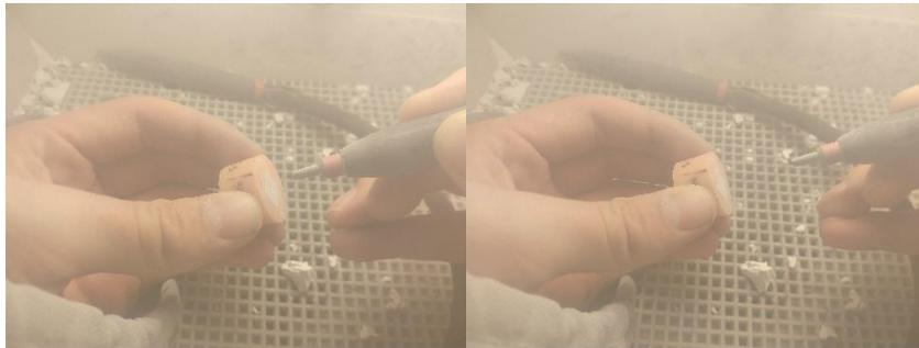
*Figure 17 – Sandblasting  $\text{Al}_2\text{O}_3$  at distances of 10 and 20 mm*
