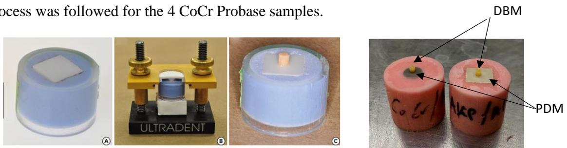
Figure 14 – Left - Example of Ultradent Shear bond mold, Right – Actual Study Samples
