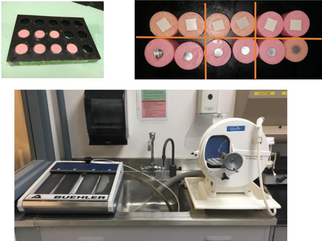
*Figure 13 – Top Left -Samples embedded with PMMA in mold, Top Right – Finished samples prior to bond, Bottom – Roll grinder and Dental Model Trimmer*
